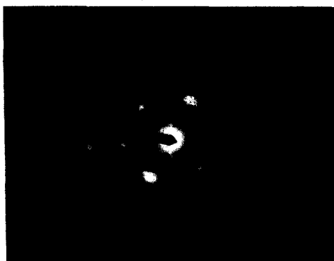
Fig. 6. Electron diffraction pattern (perpendicular to c axis) of the 2H variant of the \mu phase within the Nd-rich phase (sample M).
